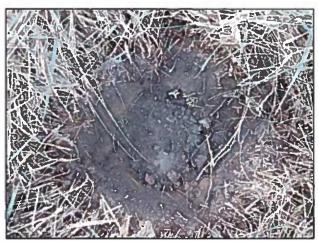
Photo 6: Test pit with evidence of previous disturbance
