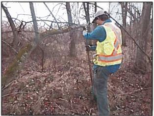
Photo 19: Test pit at 5 m intervals in wooded area
